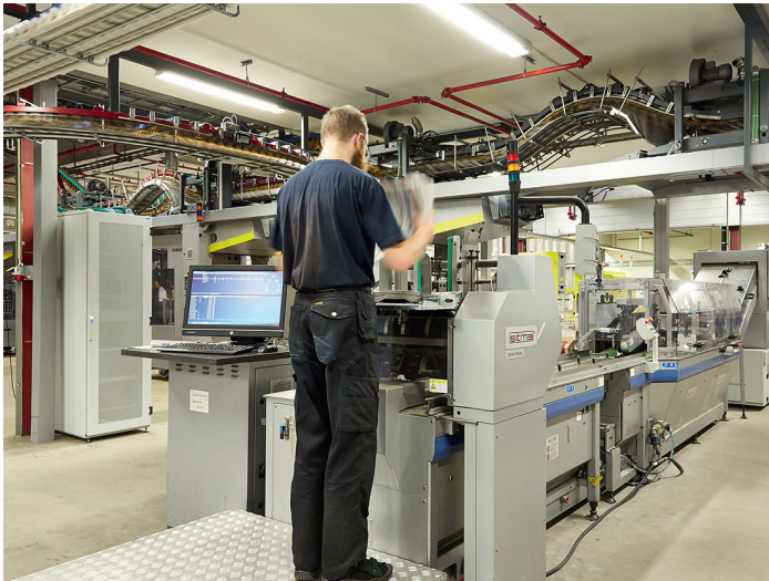
A Sitma addressing and quarterfold line is integrated into the production control system.
